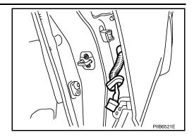
3. Remove the check link bolt from the center pillar.
