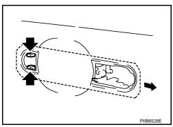
9. If equipped, disconnect the door lock assembly electrical connector.
