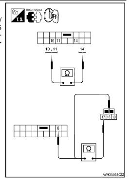
4. Check continuity between power window and door lock/unlock switch RH terminals 1, 2 and 3.
