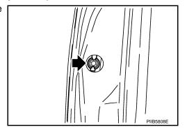
4. Pull the outside handle forward (1), while removing outside handle escutcheon (2).
