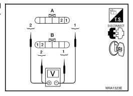
Check voltage between rear door lock actuator connector LH D202 (A) or rear door lock actuator connector RH D302 (B) terminals 1 and 2.
