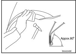
Starting from the center, hem the wheel arch gradually, using slight back and forth motion with a hemming tool.
