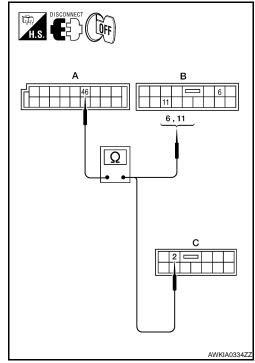
5. Check continuity between BCM connector M19 terminal 46 and ground.
