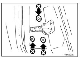
13. Slide the outside handle bracket toward the rear of the vehicle, and remove the assembly.
