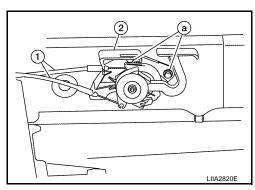
7. Remove fuel filler lid opener cable and clips from the vehicle.
