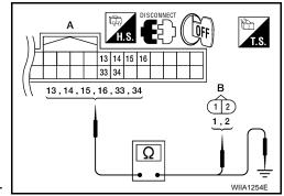
3. Check continuity between Intelligent Key unit harness connector M42 (A) terminals 13, 14, 15, 16, 33, 34 and ground.
