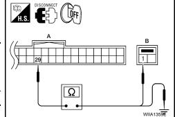
4. Check continuity between Intelligent Key unit connector M42 (A) terminal 29 and ground.
