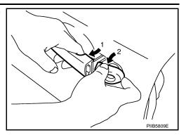
10. Pull the outside door handle out and then slide it toward the rear of the vehicle to remove.
