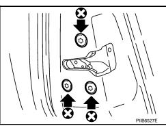
8. Slide the outside handle bracket toward the rear of vehicle, remove the outside handle bracket and the door lock assembly.
