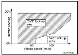
TORQUE CONVERTER CLUTCH AND SELECT CONTROL VALVE CONTROL
