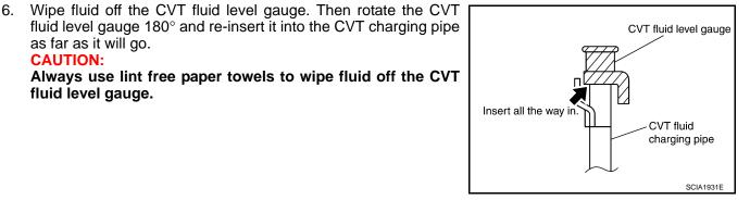
Remove the CVT fluid level gauge and check that the fluid level 7. is within the specified range as shown. If the fluid level is at or below the low side of the range, add the necessary specified NISSAN CVT fluid through the CVT charging pipe.
