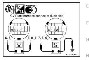
4. If NG, replace the transaxle assembly. Refer to CVT-187, "Removal and Installation (MR20DE)".
