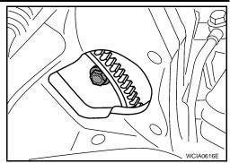
5. Put matching marks on the drive plate and torque converter alignment stud. CAUTION:
