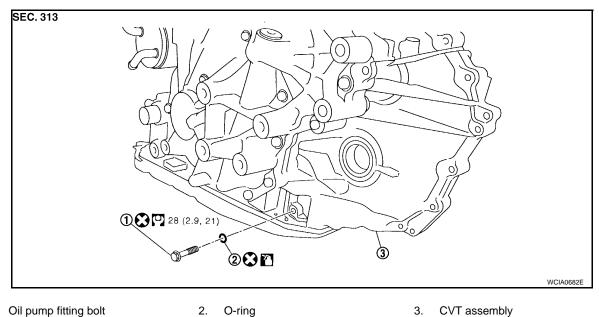
Oil pump fitting bolt 2. O-ring 1. Apply CVT Fluid. Refer to MA-13, "MR20DE".
