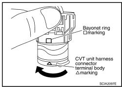
2. Rotate bayonet ring clockwise until CVT unit harness connector terminal body marking is aligned with the bayonet ring marking (linear slit) as shown.
