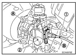
10. Remove the clip and then remove the key interlock cable from the vehicle.
