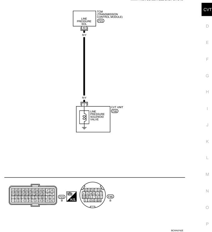
TCM TERMINALS AND REFERENCE VALUES Refer to <u>CVT-44, "TCM Input/Output Signal Reference Value"</u>.
