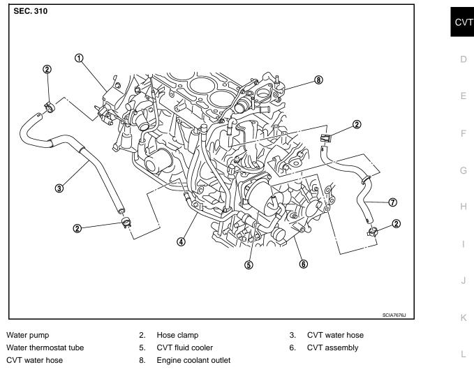
CVT Fluid Cooler Removal and Installation (QR25DE)
