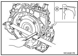
• When installing the CVT to the engine, align the matching mark on the drive plate with the matching mark on the torque converter alignment stud.
