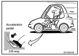
8.CHECK VEHICLE SPEED WHEN SHIFTING GEARS — PART 3
