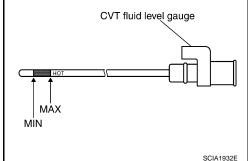
8. Install the CVT fluid level gauge to the CVT fluid charging pipe until it locks. **CAUTION:**
