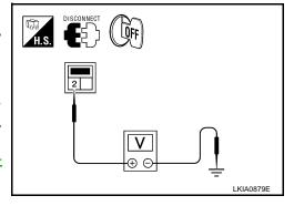
Key Switch and Ignition Knob Switch Signal Inspection (With Intelligent Key, When Mechanical Key Is Used)
