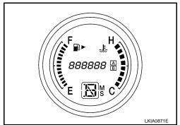
Each meter activates while pressing odo/trip meter switch.
