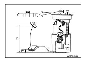
Check Fuel Level Sensor Unit and Fuel Pump Harness Check continuity at the following terminals.
