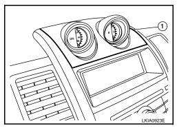
2. Disconnect the double meter assembly connector (1) and remove the double meter assembly (2).
