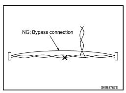
Replace the applicable harness as an assembly if error is detected on the shield lines of CAN communication line.
