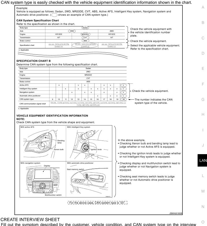
Fill out the symptom described by the customer, vehicle condition, and CAN system type on the interview sheet.
