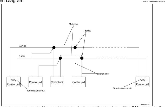
Each control unit passes an electric current to the termination circuits when transmitting CAN communication signal. The termination circuits produce an electrical potential difference between CAN-H and CAN-L. CAN communication system transmits and receives CAN communication signals by the potential difference.
