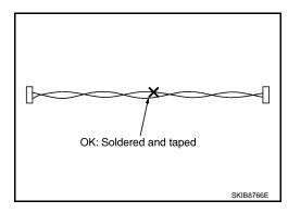
Bypass connection is never allowed at the repaired area.
