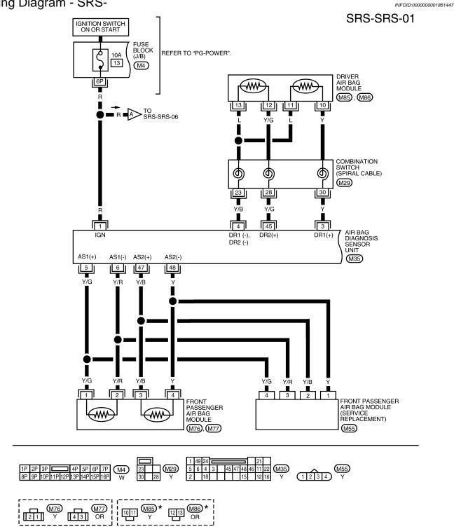
\*: THIS CONNECTOR IS NOT SHOWN IN "HARNESS LAYOUT" OF PG SECTION.
