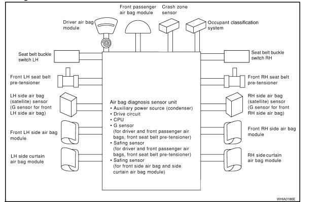
The air bag deploys if the air bag diagnosis sensor unit is activated while the ignition switch is in the ON or START position.
