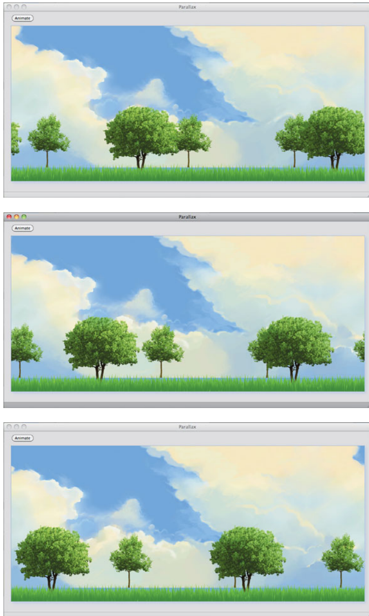
Figure 5.10 Using parallax to simulate three dimensions: From top to bottom, the bigger trees in front, moving right to left, overtake the smaller ones in back
