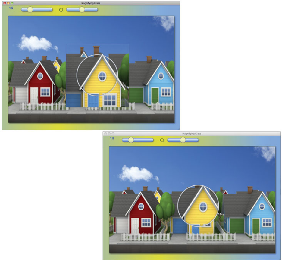
Figure 4.25 Copying magnified pixels to the magnifying glass lens. Top: unclipped; bottom: clipped
