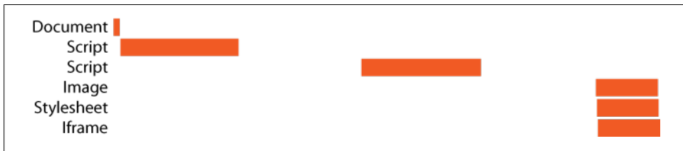
Figure 4-1. Scripts block parallel downloads
