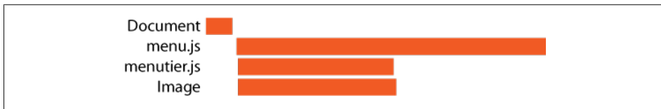
Figure 5-6. loadScripts Different Domain HTTP waterfall chart, Firefox 3
