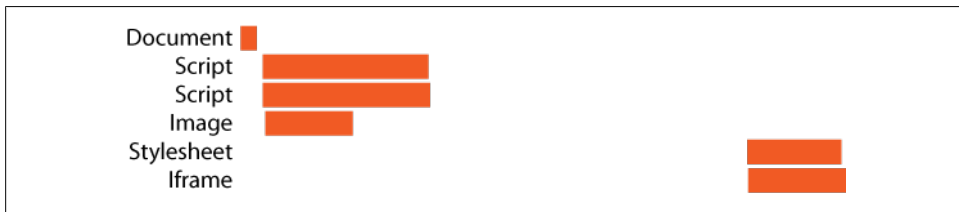
Figure 4-2. Internet Explorer 8 downloads scripts without blocking
