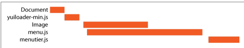
Figure 5-8. YUI Loader HTTP waterfall chart
