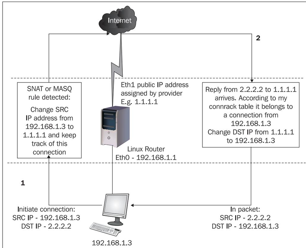
In this diagram, the computer with the IP address 192.168.1.3 tries to initiate a connection to 2.2.2.2. The packet is passed to the Linux router with the source IP address 192.168.1.3 and destination IP address 2.2.2.2.
