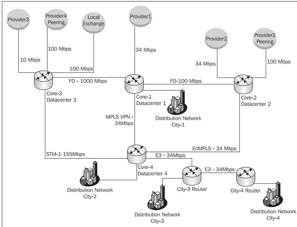
Core-1 is a router that has one FastEthernet connection to an ISP from which we buy 34Mbps of internet services. It is located in the main datacenter of this company and has a fiber optic connection at 100Mbps to Core-2 located in another datacenter. Core-1 also has a fiber optic connection at 1000Mbps (1Gbps) to Core-3.
