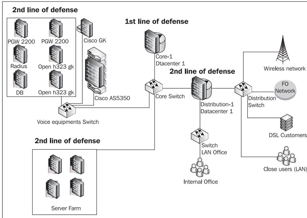
The first line of defense is Core-1, where we'll implement the firewall for all equipment in City-1. However, there can be scenarios where Core-1 is the second, third, and even fourth line of defense, depending on where the attack comes from; so we will replicate the firewall rules from Core-1 to all other core routers.
