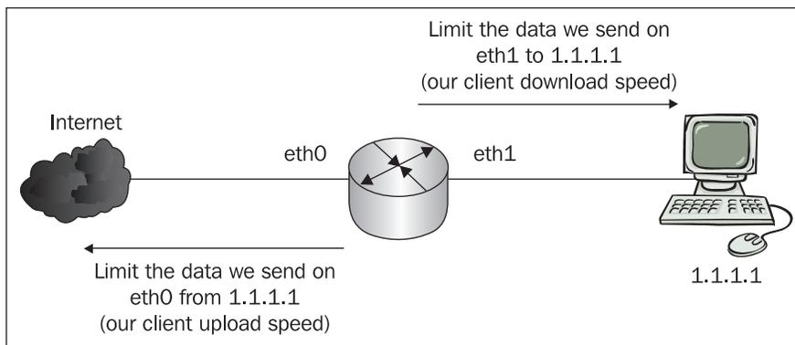
This is quite satisfying because TCP has flow control, which actually negotiates the speed of the packet flow between two communicating hosts depending on the capabilities of each host. UDP doesn't have flow control, but most of the applications that use UDP as transport protocol implement flow control within themselves.
