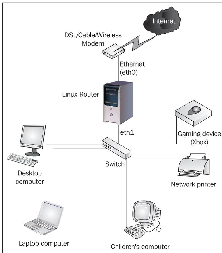
The provider usually assigns us a public IP address that can be either statically assigned or dynamically assigned using DHCP or PPPoE. Linux has support for PPPoE; this can be downloaded from <http://www.roaringpenguin.com/pppoe/>.
