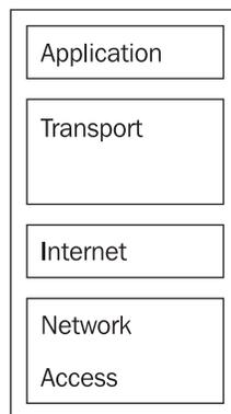
So, the layers of the TCP/IP model are: Application, Transport, Internet, and Network Access.
