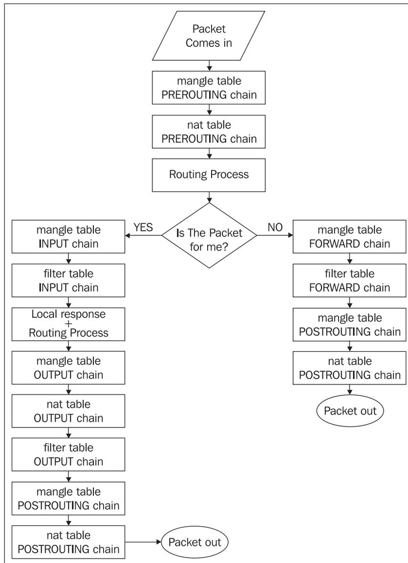
The rules in the `PREROUTING` chain of the `mangle` table are analyzed by the kernel when a packet comes in, before the routing process takes place.
