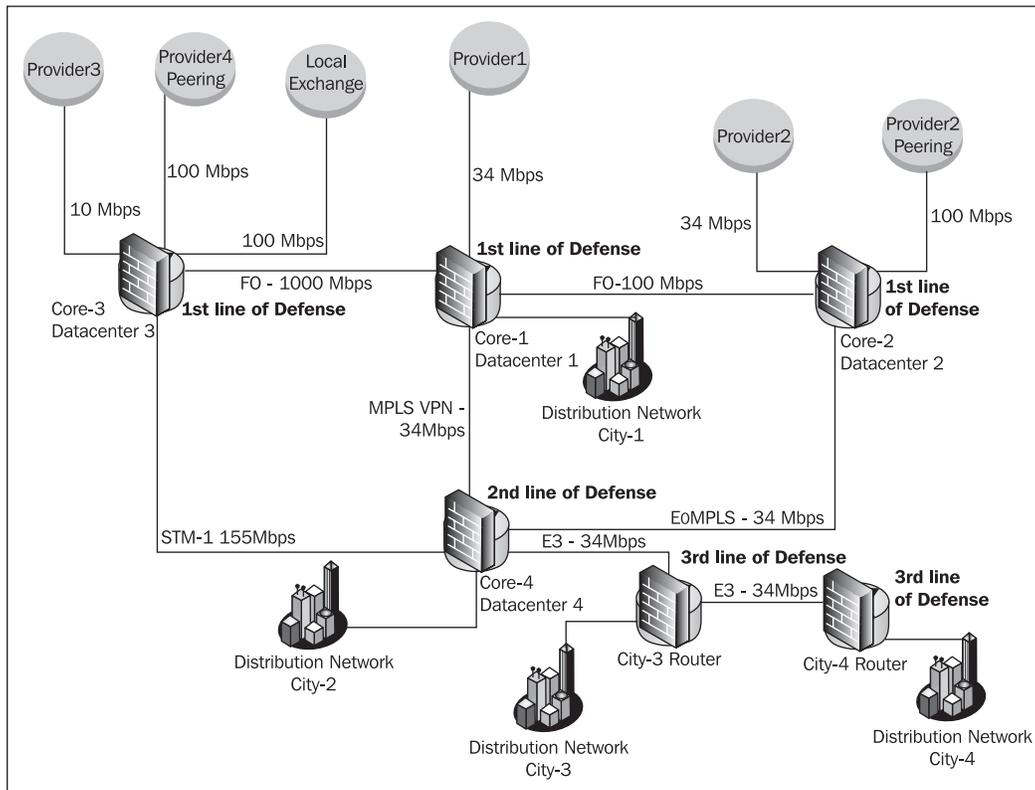
For this topology, we have to keep in mind that at any time some links may fail. At that point, the way we made the packets travel through the core links using metrics in our BGP configuration will change, and so, we have to try to unify the forward firewalls of the core routers.
