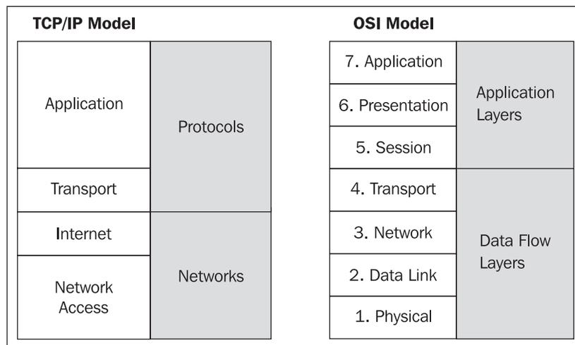
At Layer 7 of the OSI model, we find Application (HTTP, FTP, SSH, etc.). As you can see from the picture above, TCP/IP compacted OSI Layers 7, 6, and 5 into one Layer, TCP/IP Layer 4 (Application), which has the same name, but different functionality.
