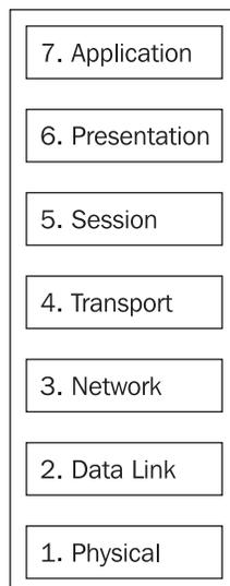
Information contained in one layer usually has headers and trailers and data encapsulated from an upper layer. **Encapsulation** is the process of placing the data from an upper layer between headers and trailers so that when data is received by a layer, after it is analyzed, the protocol at that layer removes the headers and trailers and gives the data to the upper layer in the format that the upper layer understands.
