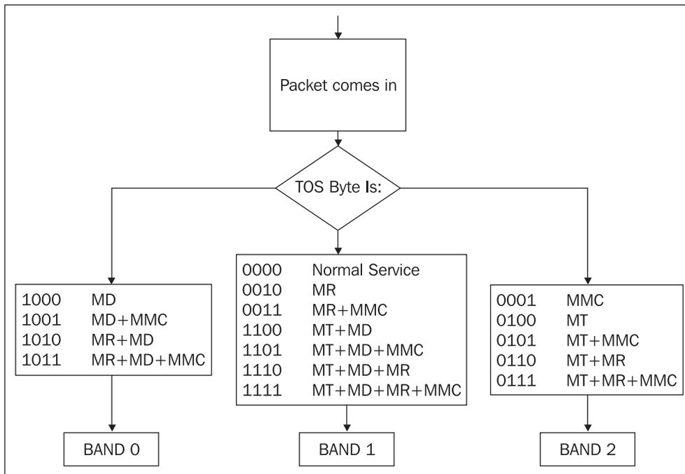
This means that, by default, Linux is smart enough to prioritize traffic according to the TOS bytes. Usually, applications like Telnet, FTP, SMTP modify the TOS byte to work in an optimal way. We will see later in this book how to optimize the traffic ourselves.
