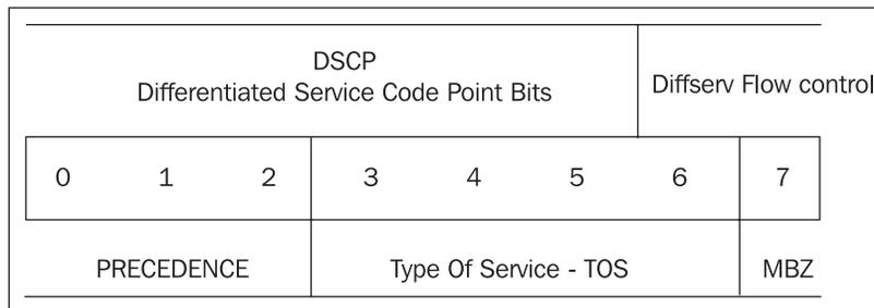
iptables has the DSCP target that can be used to alter the DSCP bits. The options can be found using `--help` with the DSCP target.
