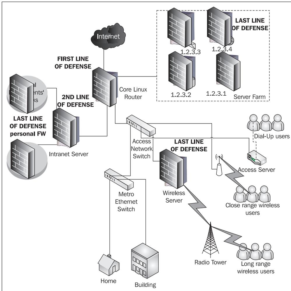
From a security point of view, the core router is the first line of defense. The first line of defense should stop all attacks coming from outside. However, if the firewall at the core router fails, then the firewall on each server is responsible for the security of that server.
