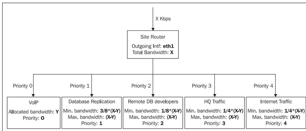
To differentiate these services we will mark packets in the `mangle` table in the `POSTROUTING` chain for every service, using the `MARK` target of iptables (module `ipt_MARK`).
