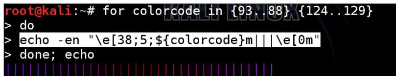
How does this work? Well we need to discuss some of the basic text formatting control sequences. These control the style of the text, which includes properties such as emboldening text, underlining, and inverting the terminal printing. The control sequences are as follows:
